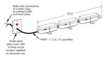
**Step 2:** Position Light extensions according to design layout. Connect the module at the end of the the power set to the first module of the first light extension by plugging the quick-connects together. Plug and play connections between module sets allow for fast and easy installation.
