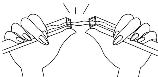
**Step 4:** Pull sets of wires from open tube ends and cut with wire cutters. Be sure to leave enough wire to connect it to the next tube.
