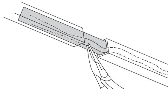
**Step 5:** Use a sharp knife or cutter to cut off the extra length of backing board that is extending out of the end of the cut tube. Pull the board out a little further to cut it to make room for the end cap to fit inside the tube.
