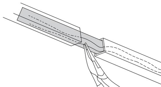
**Step 5:** Use a sharp knife or cutter to cut off the extra length of backing board that is extending out of the end of the cut tube. Pull the board out a little further to cut it to make room for the end cap to fit inside the tube.
