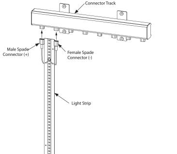
**Step 2**: The light strips have pre-drilled holes for mounting screws placed every 12 inches along each strip. Position each strip so it is centered between connectors and the top edge is close to the bottom edge of the Connector Track. Secure Light Strips with fasteners appropriate for the type of mounting surface, ie: wood screws for wood (by others).
