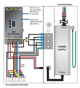
ADNM-150-2-5-12-DIN-2 100-277V AC / 12V DC, 120W /2 CIRCUITS X 5A ADNM-240-2-4-24-DIN-2 100-277V AC / 24V DC, 192W /2 CIRCUITS X 4A
