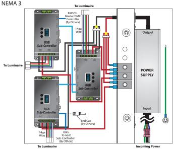
ADNM-240-3-5-12-DIN 100-277V AC / 12V DC, 180W /3 CIRCUITS X 5A ADNM-320-3-4-24-DIN 100-277V AC / 24V DC, 288W /3 CIRCUITS X 4A
