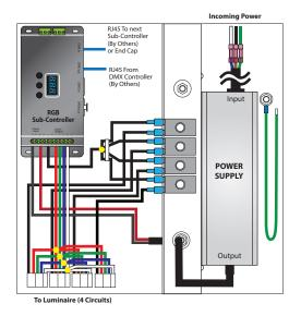
ADNM-240-3-5-12-DIN-3 100-277V AC / 12V DC, 180W /3 CIRCUITS X 5A ADNM-320-3-4-24-DIN-3 100-277V AC / 24V DC, 288W /3 CIRCUITS X 4A
