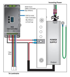
ADNM-60-1-5-12-DIN\* 100-277V AC / 12V DC, 60W /1 CIRCUIT X 5A ADNM-90-1-4-24-DIN\* 100-277V AC / 24V DC, 90W /1 CIRCUIT X 4A \*Not suitable for RGBW
