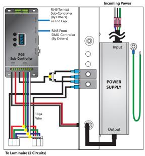
ADNM-80-1-5-12-DIN 100-277V AC / 12V DC, 60W /1 CIRCUIT X 5A ADNM-120-1-4-24-DIN 100-277V AC / 24V DC, 96W /1 CIRCUIT X 4A **BOX SIZE:** 12" X 12" X 4" NEMA 3
