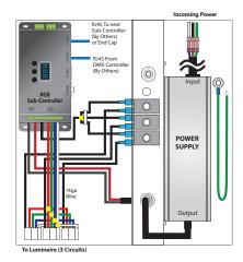
ADUL-150-2-5-12-DIN-2 100-277V AC / 12V DC, 120W /2 CIRCUITS X 5A ADUL-240-2-4-24-DIN-2 100-277V AC / 24V DC, 192W /2 CIRCUITS X 4A
