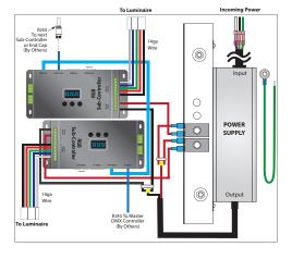
ADUL-80-1-5-12-DIN 100-277V AC / 12V DC, 60W /1 CIRCUIT X 5A ADUL-120-1-4-24-DIN 100-277V AC / 24V DC, 96W /1 CIRCUIT X 4A
