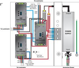
ADUL-240-3-5-12-DIN 100-277V AC / 12V DC, 180W /3 CIRCUITS X 5A ADUL-320-3-4-24-DIN 100-277V AC / 24V DC, 288W /3 CIRCUITS X 4A
