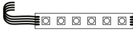
TPL-I-LEAD-4-C LEAD/END 24" standard 4 conductor 22AWG lead wire factory attached to one end of tape
