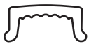
WW-TC-XX-8 XX = BK (Black), GY (Gray), CL (Clear), BZ (Bronze) Top Cover Wire Way lens, 8' length
