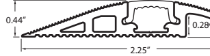
WW-CE-XX-8 XX = BK (black), GY (gray) Carpet to Edge Base and Cover Combo, 8' length
